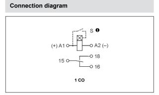
• The control terminal S is activated by connection to A1 terminal via the external control contact S.
