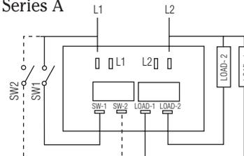
Note: For ease of wiring, L1 and L2 each have two tabs.
