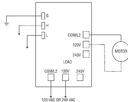
**Caution:** 19MR contacts are powered contacts. When power is applied to the 19MR controller, power may be present on relay output connections. Output voltage will be same as input voltage.
