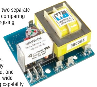
**Intrinsically Safe Controls** are solid state controls which limit current and voltage to a level incapable of igniting flammable gasses, vapors or dust. They can be used as conductivity liquid level controls or with dry contact devices such as Gems Flow and Level Switches or other non voltage storing or producing devices.
