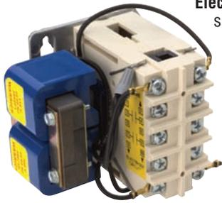
**Electromechanical Controls** employ a simple series circuit which includes the transformer, relay coil, electrode probes and the liquid media being monitored. When liquid contacts both the reference and set point electrode probes, current flows through the liquid media which in turn energizes the relay coil and mechanically changes the output contacts state.
